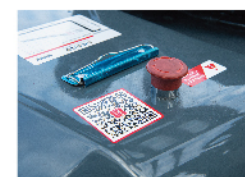
Emergency power-off switch is equipped as standard to ensure safety in case of emergency;
