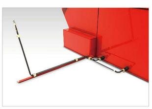
Molding steel pipe is used for oil suction pipe improving safety degree largely.
