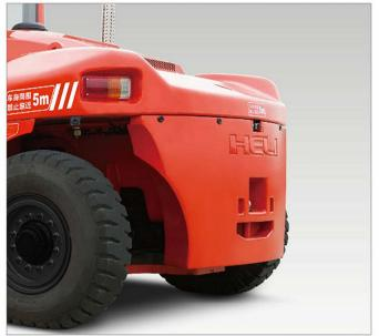
Counter weight no air channel design Special cooling system layout and temperature control system are adopted on G series truck. rear counter weight has no air channel and counter weight use ratio is increased and thus truck service weight is reduced.
