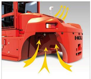
Optimal designed channel Optimal designed radiator and channel make cooling system have small resistance, avoid air flowing back effectively and improve cooling efficiency.
