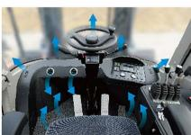
Temperature control system through multiple channel Fully sealed cab controls temperature in the cab high efficiently and multiple channels cross ventilation keep the temperature in the cab stable. winter.
